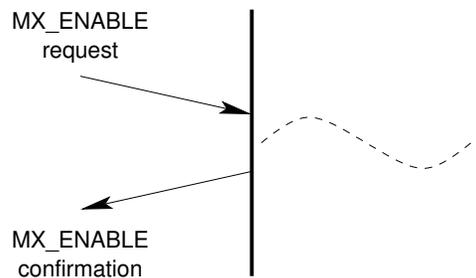
Figure 3.6: *Message Flow: Successful Enable Service*
