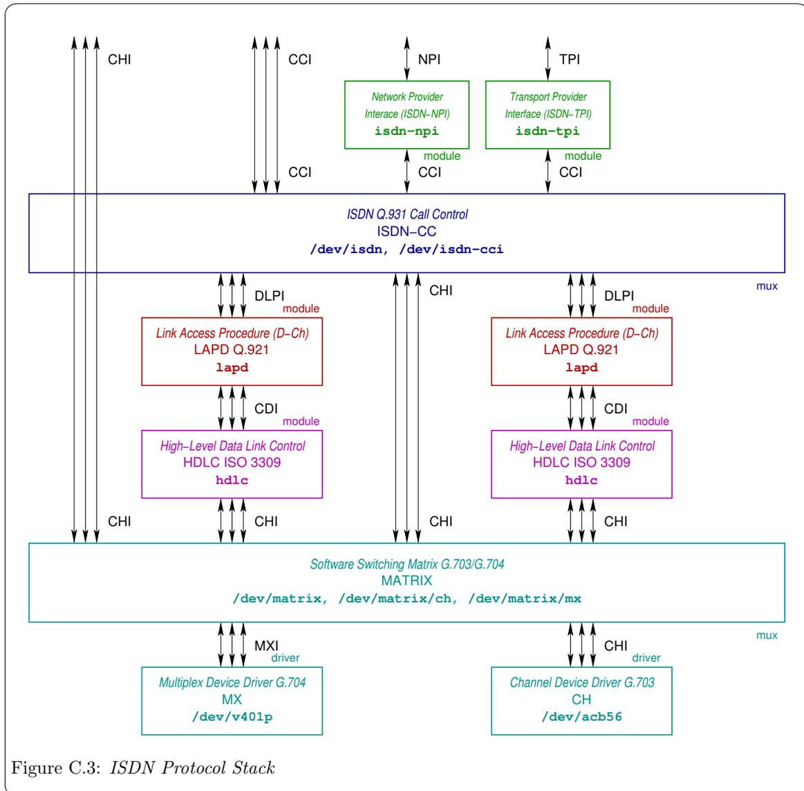
Figure C.3: ISDN Protocol Stack
