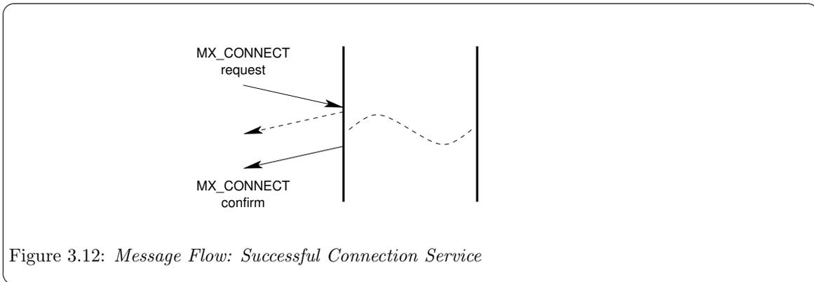
Figure 3.12: *Message Flow: Successful Connection Service*
