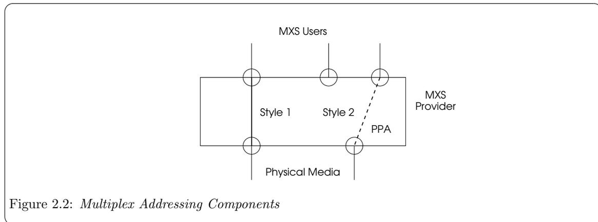
Figure 2.2: *Multiplex Addressing Components*
