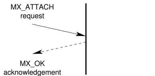
Figure 3.4: *Message Flow: Successful Attachment Service*
