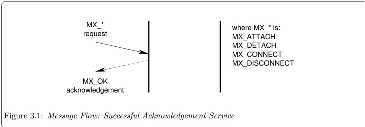
Figure 3.1: Message Flow: Successful Acknowledgement Service
