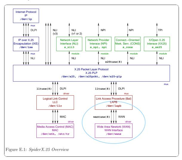
The SpiderX.25 stack implementation differs from the OpenSS7 X.25 Networking one in several fundamental ways:
