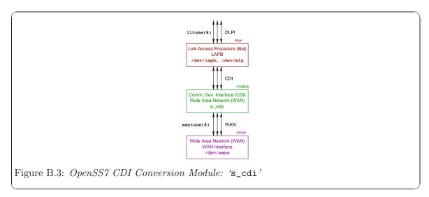
The 's\_cdi' pushable *STREAMS* module accepts a Wide Area Network (WAN) Interface at its lower service boundary and provides a Communications Devce Interface (CDI) at its upper service boundary.
